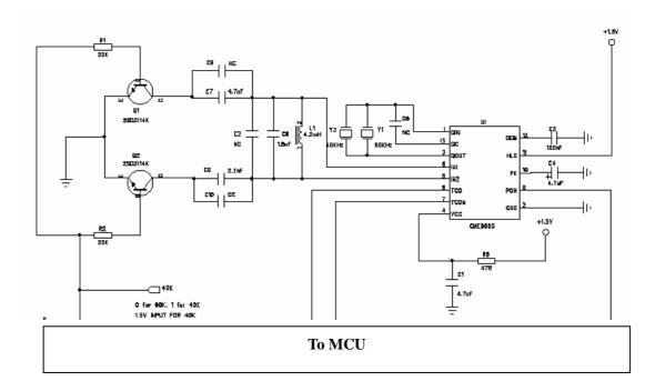
The MCU is responsible for the control of switch between the two frequencies, controlling the power on (PON) of the receiver IC as well as analyzing the pulses that are provided as output from the CME6005 (TCO or TCON)
